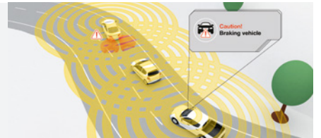
Emergency Electronic Brake Lights (EEBL)
