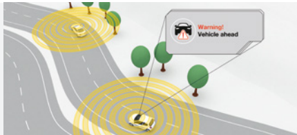
Forward Collision Warning (FCW)
